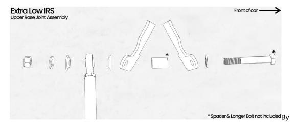
moving the fixing point outside of the cradle housing it allows more free movement and stops the drop link binding against the main cradle.
