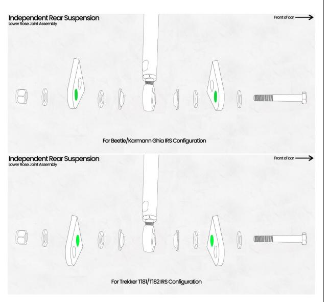
Please refer to the above diagrams to ensure the assembly is positioned in the correct fixtures, highlighted in green demonstrates the correct eyelet to use for either T1 Beetle/T14 Karmann Ghia and also for Trekker T181/T182.
