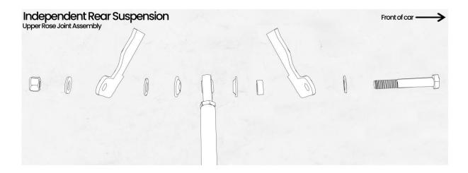
Position the spacer to the REAR SIDE of the cantilever, this will mean your pushrod sits closer to the front of the car, this is the correct alignment in most cases.
